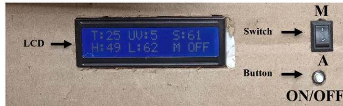
**Figure 34.** LCD screen displaying sensor metrics in manual mode with system turned OFF
