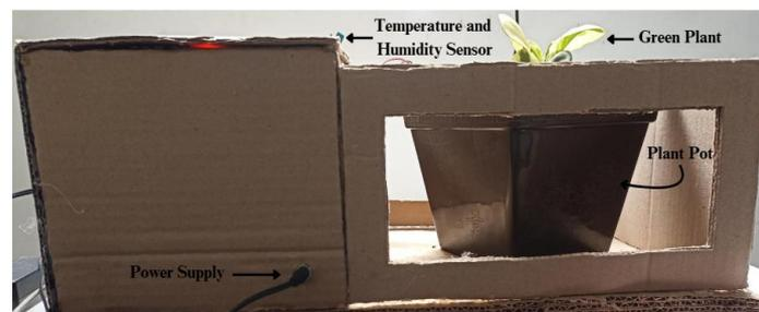
**Figure 35.** Side view of the physical implementation of the system
