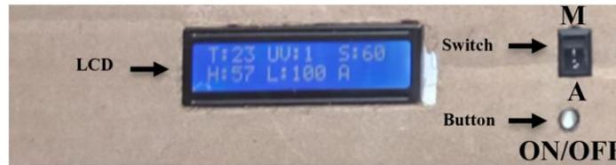
Figure 31. LCD screen displaying sensor metrics and automatic mode
