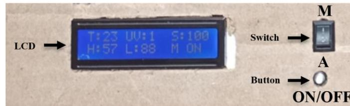
**Figure 33.** LCD screen displaying sensor metrics in manual mode with system turned ON
