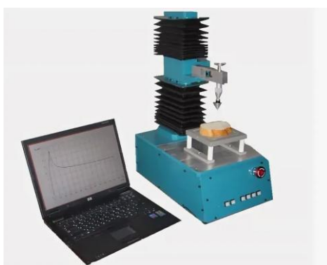
Figure 4. An image of the Structurometer ST-2 device
