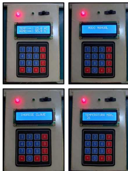
Figure 16. Operation of the Electronic Circuit for the Automatic Irrigation System
