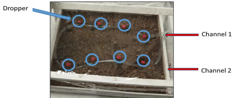
Figure 18. Location of Irrigation Channels in the Automated Irrigation System
