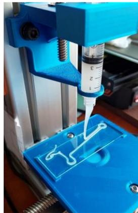
**Figure 3. DIW printing onto bottom float glass**
