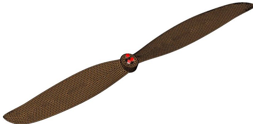
Figure 4. 3D design of plastic propeller with three gates location
